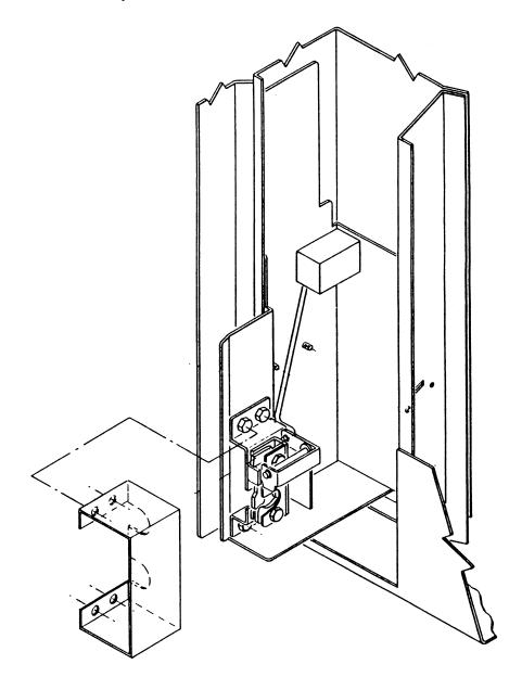
To install the latch baffle (360,010,210.03), remove the four (4) 5/16-18 nuts securing the latch mount to the main bracket. Position the baffle on the four (4) thread studs as shown and reinstall the nuts.
